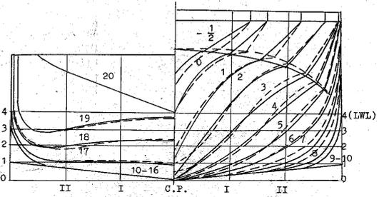
Figure 8. The comparison of the hull shapes of R69 with the hull shapes of variant 2 from developable surfaces
