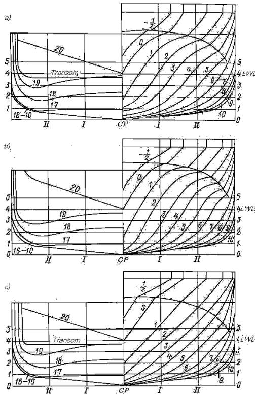
Figure 7 The hull shapes of R69
