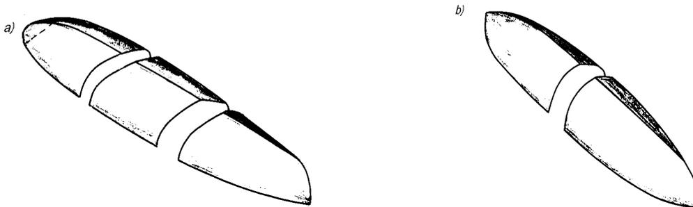
Figure 4. Formation of ship shapes from developable surfaces. a) – the hull shapes with a middle body; b) - the hull shapes without a middle body.
