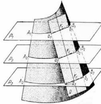
Figure 2. Cuts of polyparametrical developable surfaces by parallel planes
