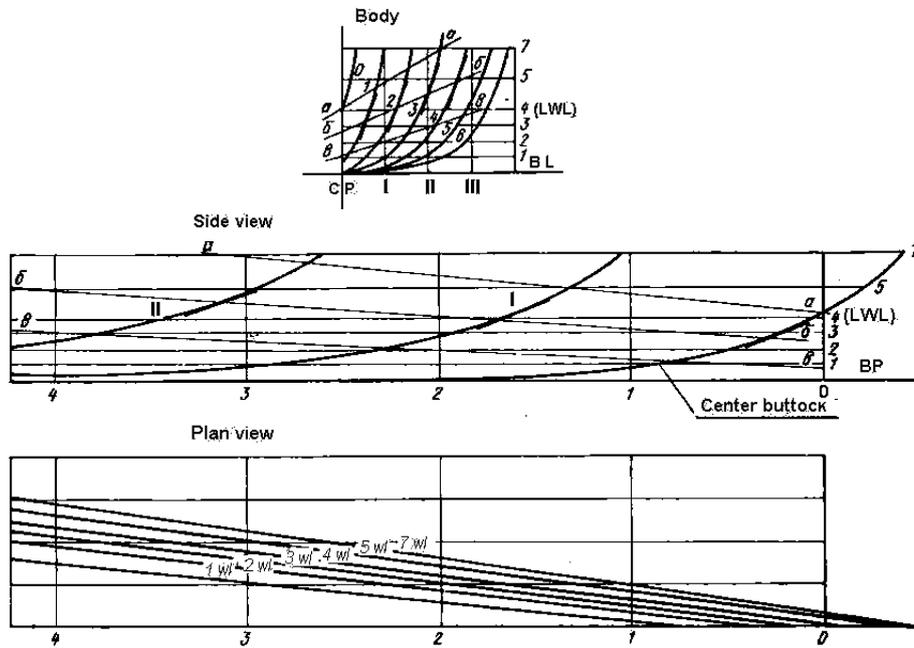
Figure 3. The construction of ship hull shapes from developable surfaces.
