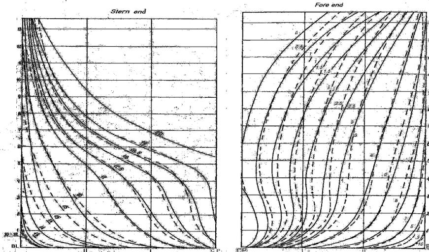
Figure 5. The afterbody and forebody of ship with a bow bulb
