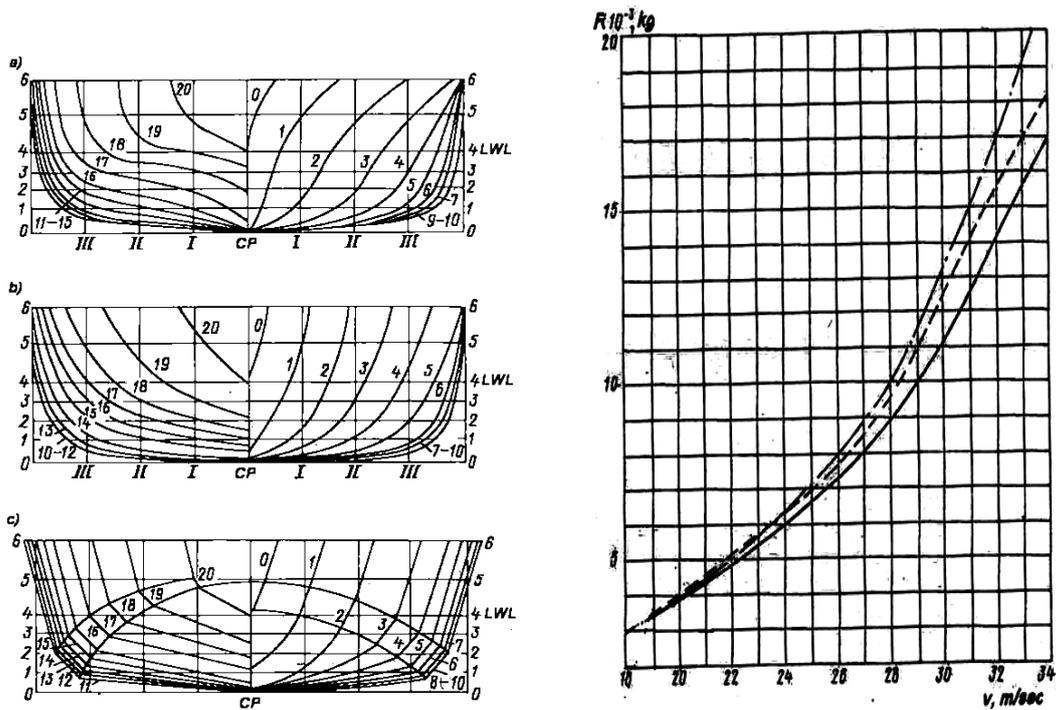
Figure 6. Hull shapes of a river vessel such as "«Rodina" and the comparative resistance curves of these variants of hull shapes a) – initial variant with usual shapes; b) – shapes with developable skin; c) – "simplified" hull shapes. The upper curve is the resistance of variant c; the lower curve is resistance of variant b; the middle curve is resistance of variant a
