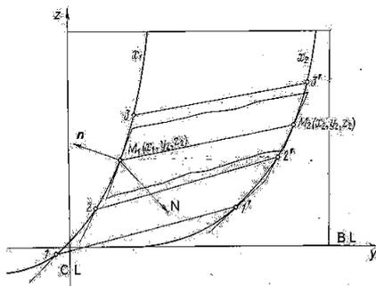
Figure 10. Normal to a frame  $n$  and a tangent plane with normal to it  $N$ .
