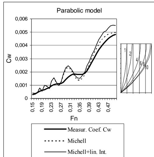
Figure 3. Comparison of the wave resistance coefficients with and without the line integral (Wigley parabolic model).
