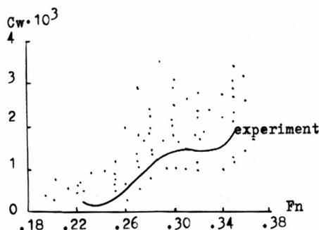
Figure 2. A collection of computer predictions of wave resistance for the Series 60 hull using linearized theory taken from the two workshops differ only in their method of solution (A.Musker [1989], figure 1).
