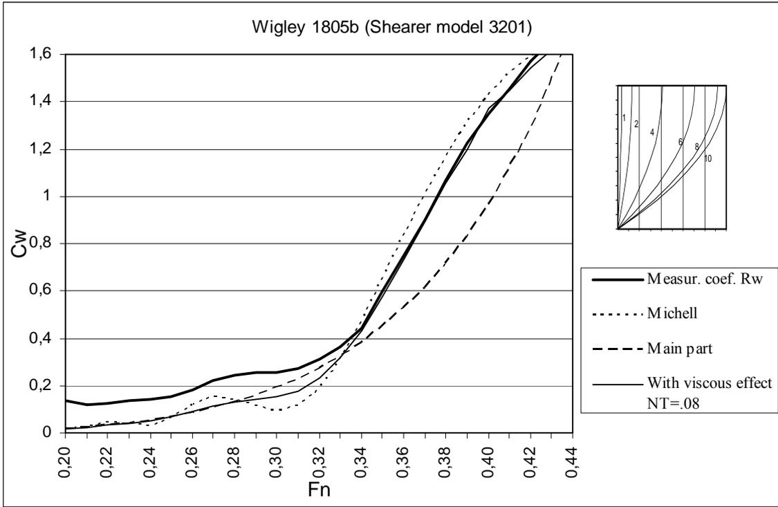
Figure 3A. Wave resistance coefficients of Wigley model 1805b.
