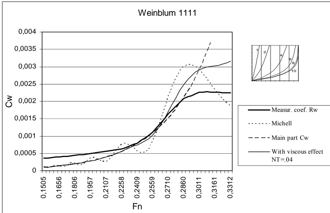
Figure 17A. Wave resistance coefficients of Weinblum model 1111.
