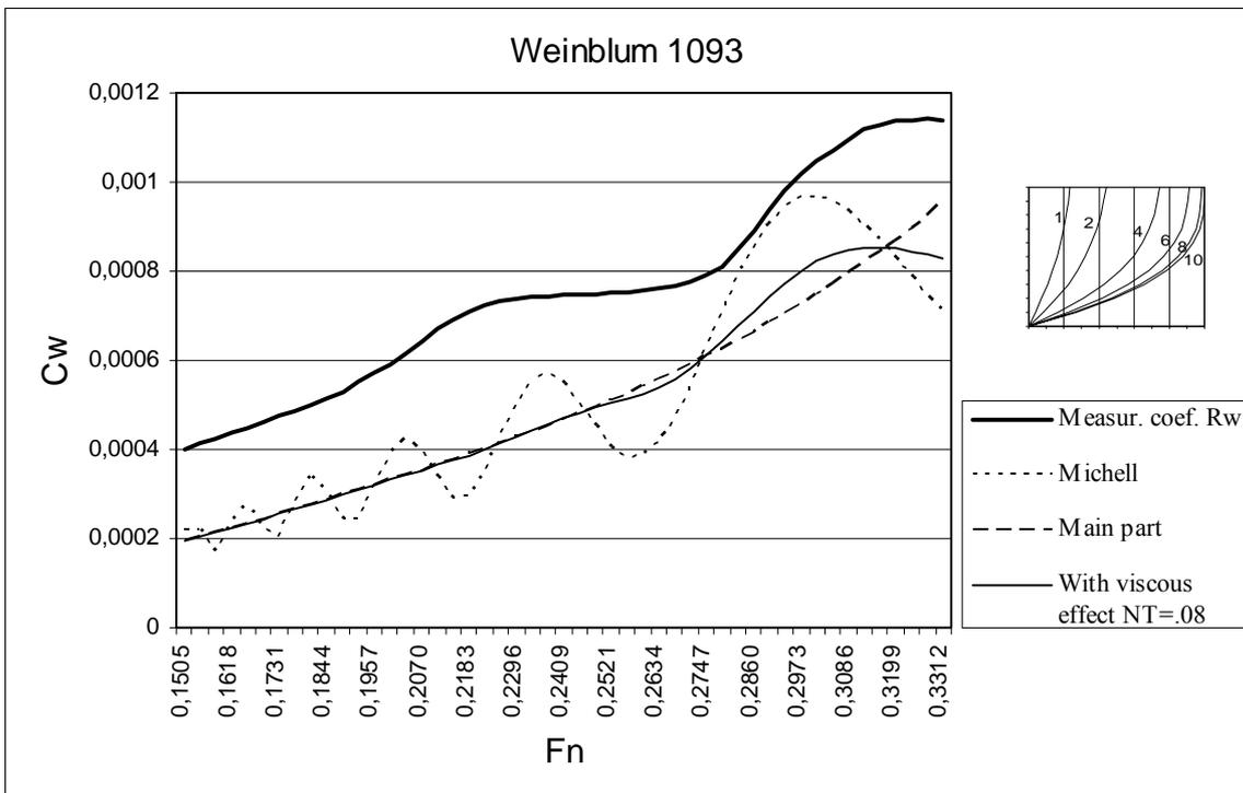
Figure 12A. Wave resistance coefficients of Weinblum model 1093.
