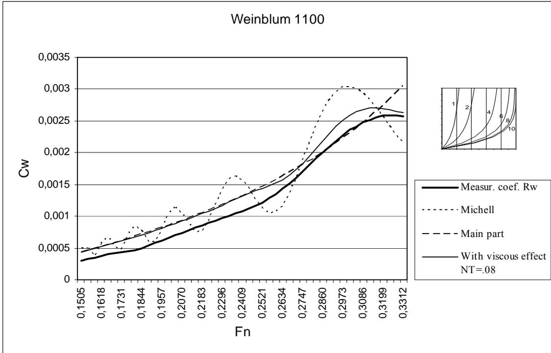
Figure 15A. Wave resistance coefficients of Weinblum model 1100.
