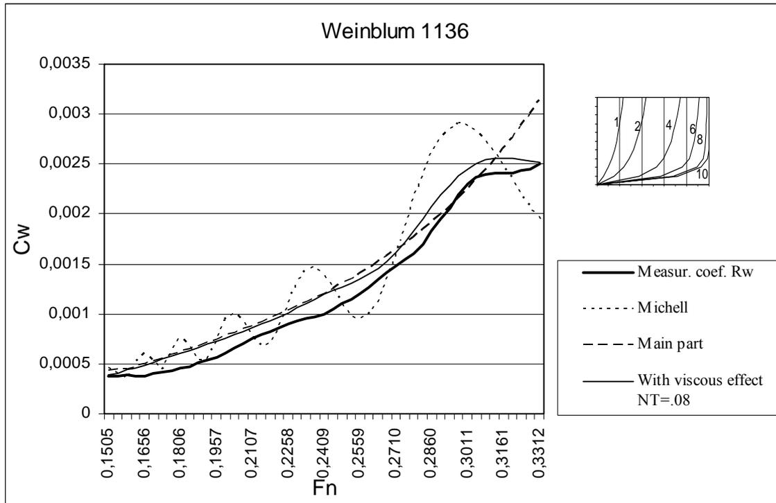
Figure 21A. Wave resistance coefficients of Weinblum model 1136.
