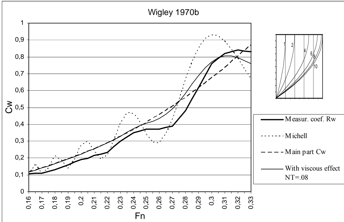
Figure 6A. Wave resistance coefficients of Wigley model 1970b.
