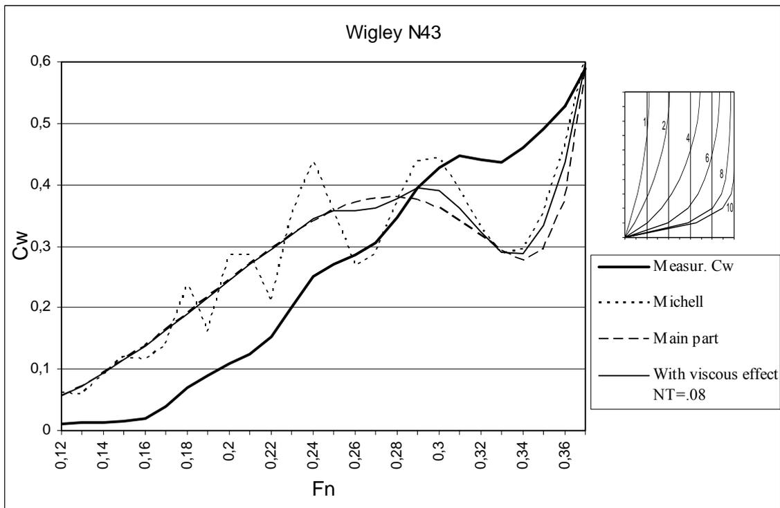
Figure 8A. Wave resistance coefficients of Wigley model N43.
