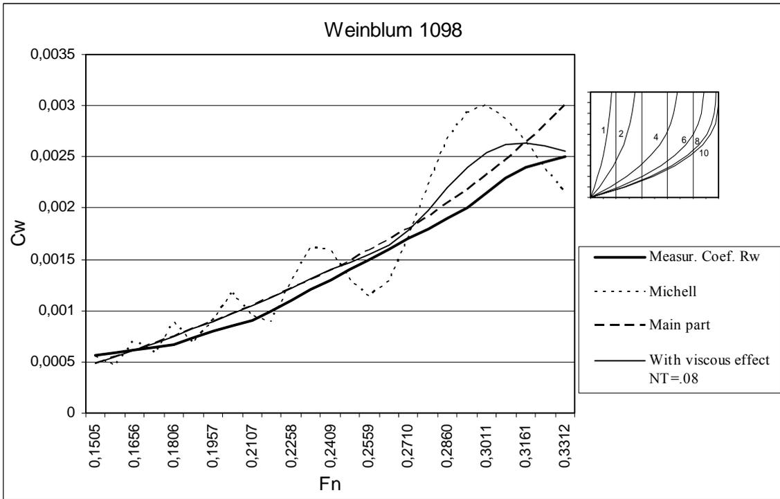
Figure 14A. Wave resistance coefficients of Weinblum model 1098.
