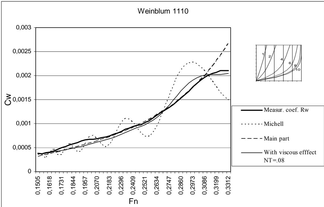
Figure 16A. Wave resistance coefficients of Weinblum model 1110.
