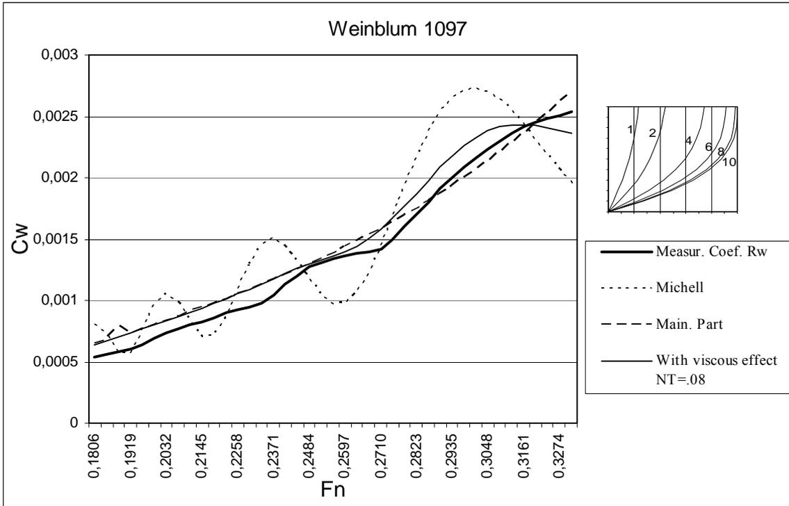
Figure. 13A. Wave resistance coefficients of Weinblum model 1097.
