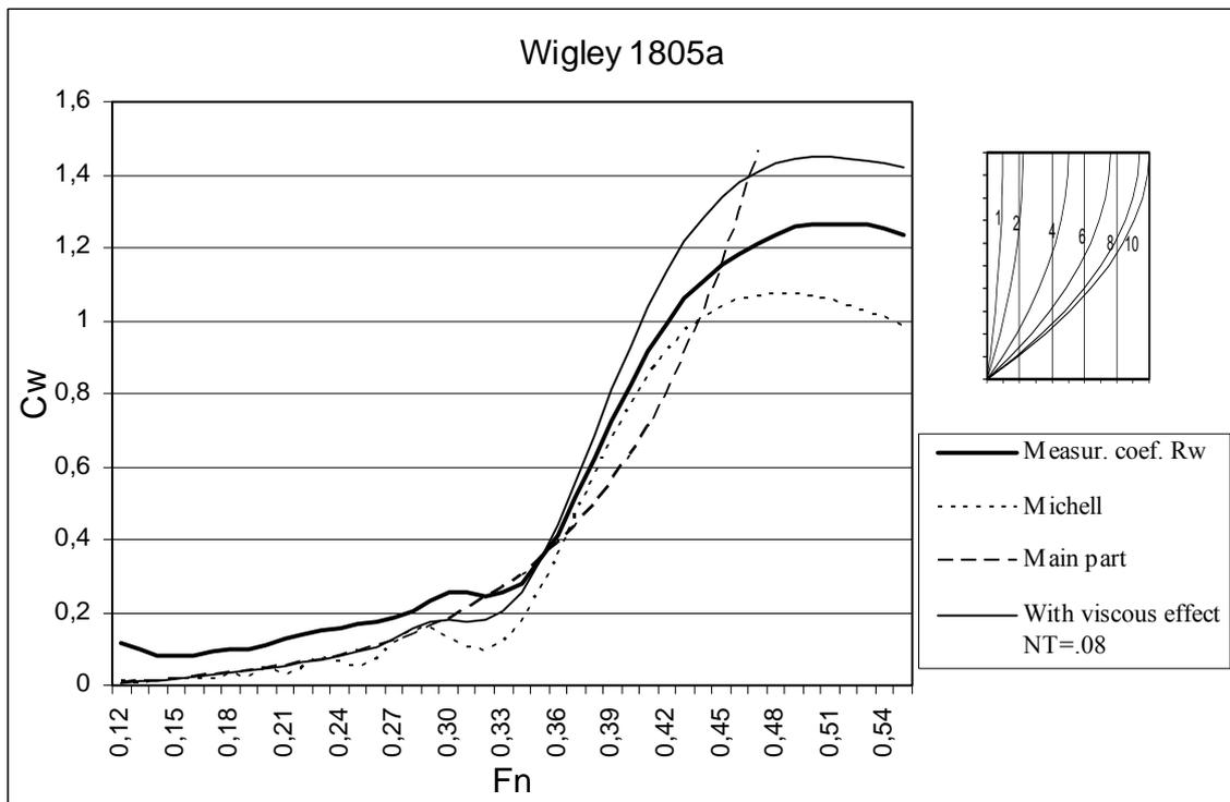
Figure 2A. Wave resistance coefficients of Wigley model 1805a.
