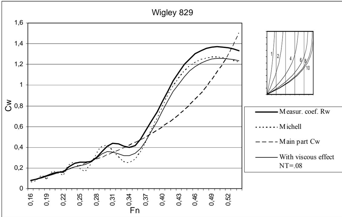
Figure 1A. Wave resistance coefficients of Wigley model 829.
