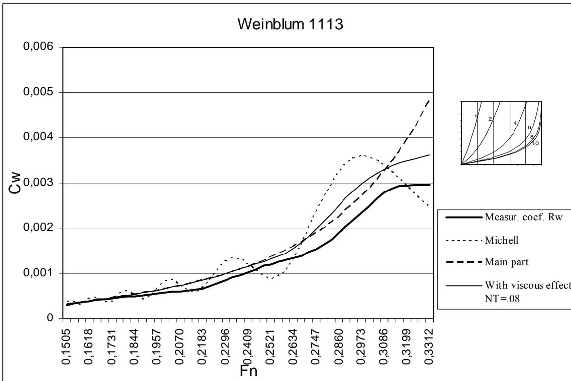
Figure 19A. Wave resistance coefficients of Weinblum model 1113.
