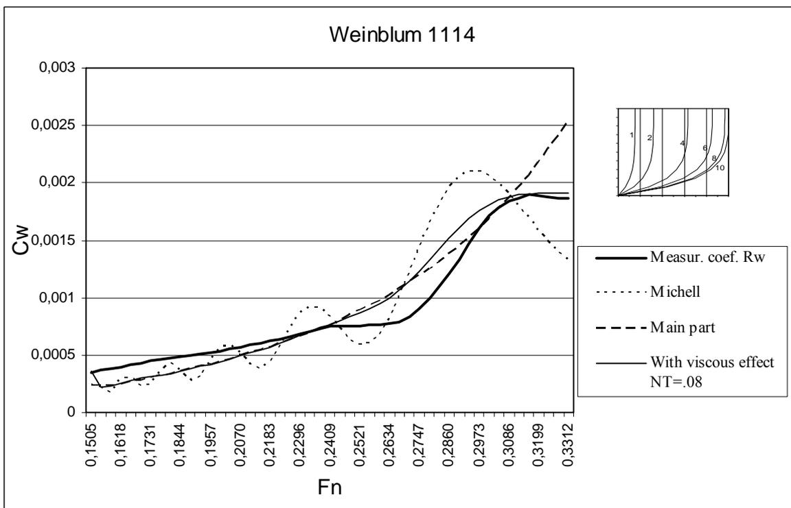
Figure 20A. Wave resistance coefficients of Weinblum model 1114.
