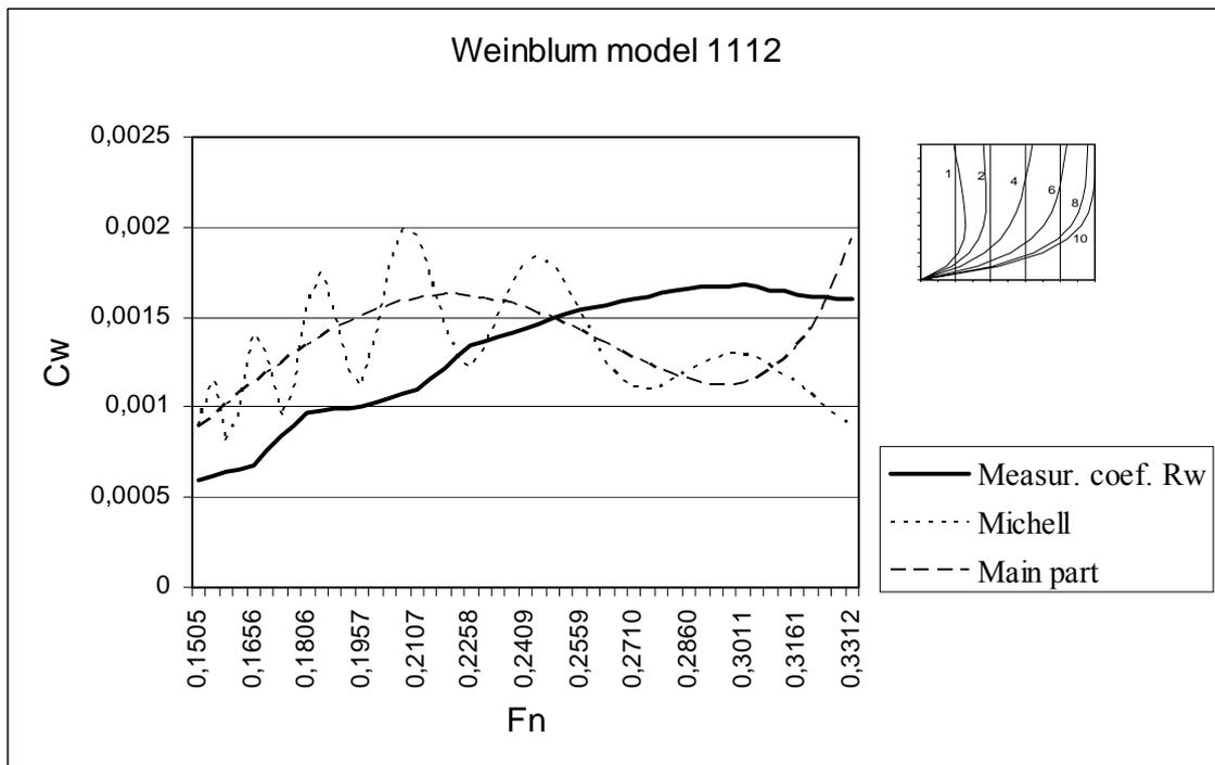
Figure 18A. Wave resistance coefficients of Weinblum model 1112.
