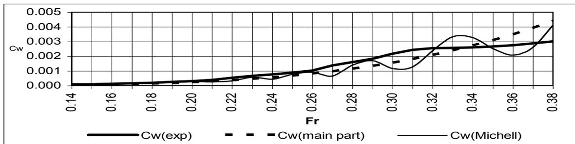
Fig. 5 Calculated and experimental of the wave resistance coefficients of model "Rodina"
