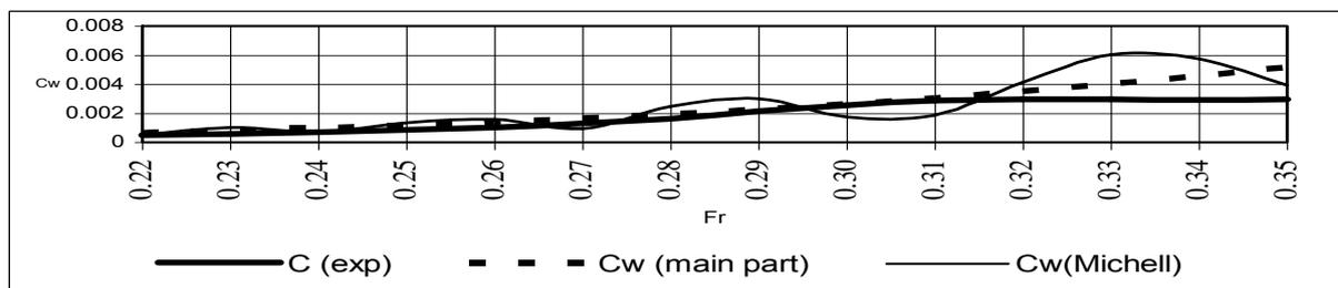
Fig. 4. Calculated and experimental coefficients of the wave resistance of model "Sevan"
