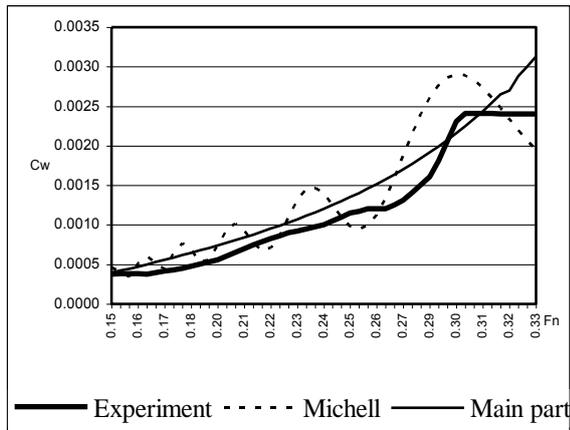
Fig. 11 Comparison of Michell's curves and residual
