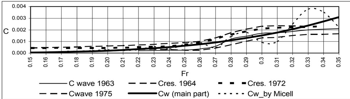
Fig. 3. Calculated and experimental coefficients of the wave and residual resistance of Todd's model
