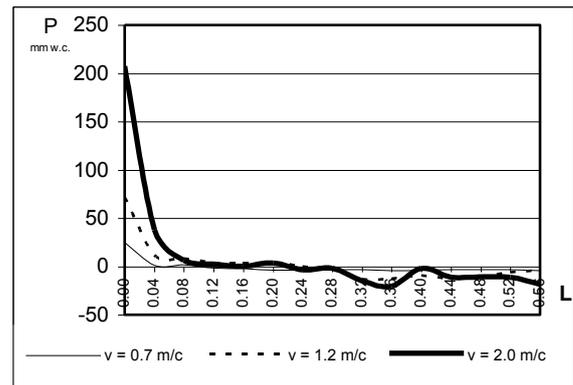
Fig. 10 The distribution of pressure on model on  $t = 0.1m$ , draft 0.2 m (the towing tank of NSAWT)
