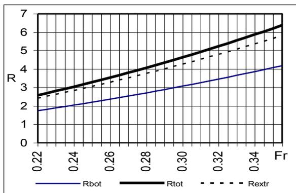
Fig. 6. Friction resistance of Todd's model
