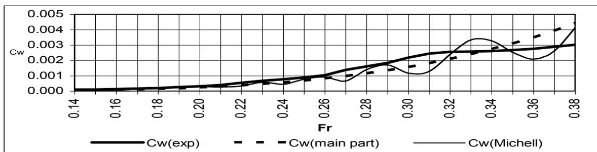
Fig. 5 Calculated and experimental of the wave resistance coefficients of model "Rodina"
