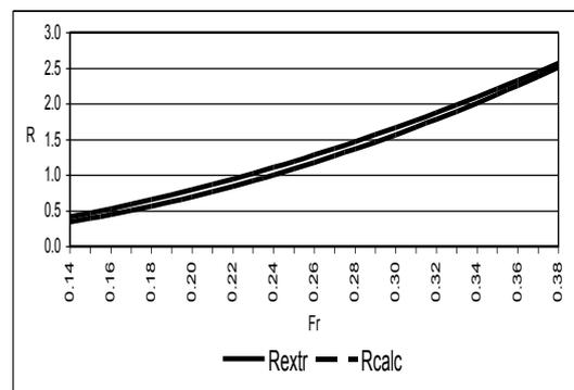
Fig. 8. Friction resistance curves obtained by extrapolator and by the integral relation of Weinblum's 1100 model
