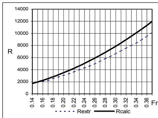
Fig. 7. Friction resistance of vessel "Rodina"
