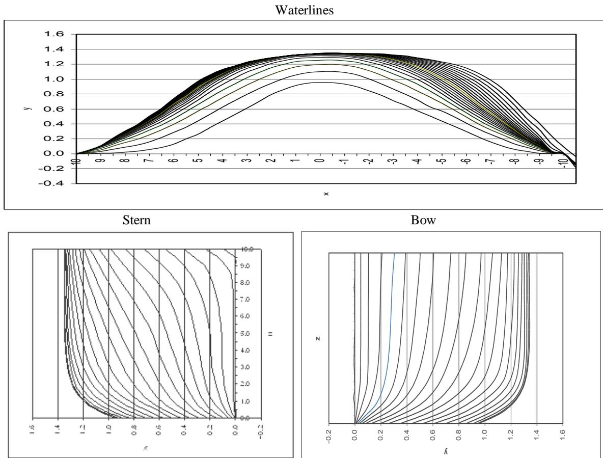
Fig. 1 Body plans under the main waterline of Todd's model 0.6
